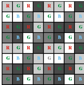
Figure 2. SVE Color Filter array [2]
