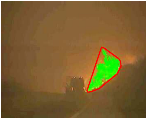
Fig. 4. Illustration of the convex hull (red line) used to evaluate the boundary roughness of the blob.
