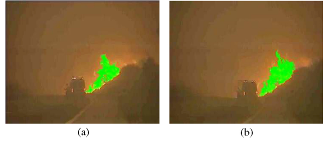
Fig. 3. Illustration of the change in fire pixel area from frame to frame. (a) Fire area = 1692 pixels. (b) Fire area = 2473 pixels.
