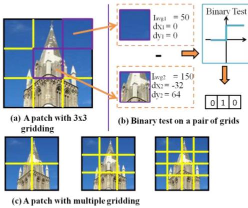
Fig. 1. Illustration of LDB extraction. (a) An image patch is divided into  $3 \times 3$  equal-sized grids. (b) Compute the intensity summation ( $I$ ), gradient in  $x$  and  $y$  directions ( $d_x$  and  $d_y$ ) of each patch, and compare  $I$ ,  $d_x$ , and  $d_y$  between every unique pair of grids. (c) Three-level gridding (with  $2 \times 2$ ,  $3 \times 3$ , and  $4 \times 4$  grids) is applied to capture information at different granularities.
