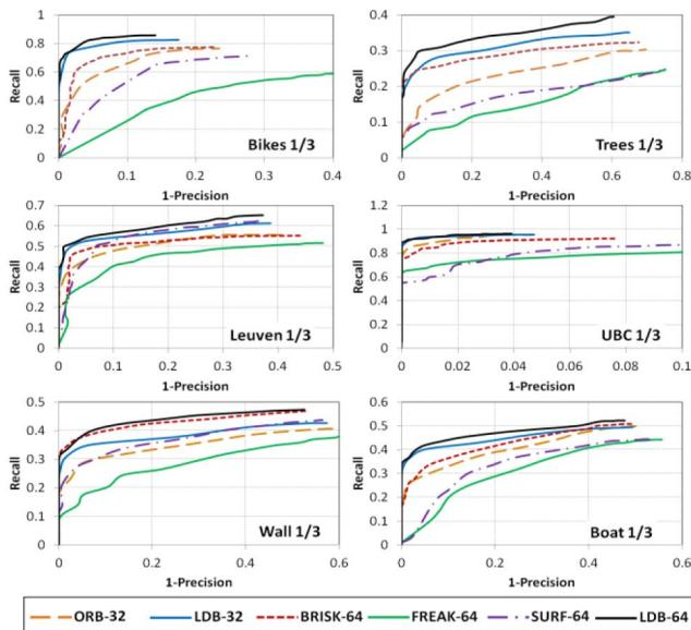
Fig. 4. Recall versus 1-Precision curves obtained by LDB, ORB, BRISK, FREAK, and SURF for image pairs 1/3 of VggAffine data set.
