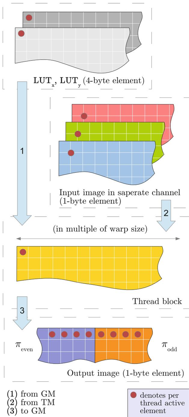
**Fig. 9** Implementation of the data interpolation procedure in CUDA
