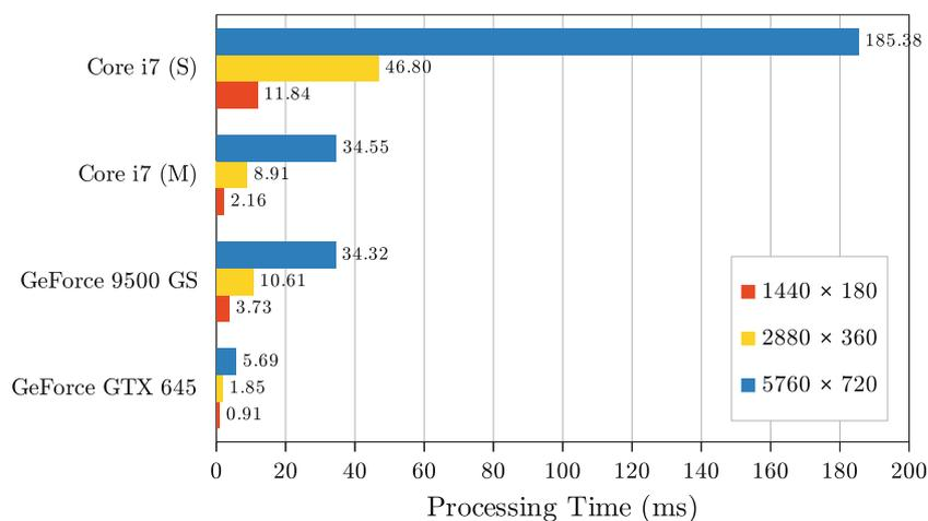
**Fig. 14** The breakdown of the GPU data interpolation kernel processing speed for a 24-bit image
