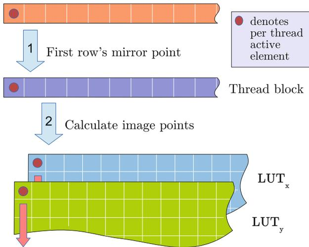
**Fig. 7** The sequence design of the GPU kernel of stage three in the mapping procedure
