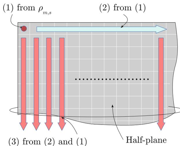
**Fig. 4** A systematic procedure is used to solve all the  $\rho_m$  in the half-plane using  $\rho_m, s$ . The first pixel (red dot) is solved from  $\rho_m, s$ , then the first row (blue arrow) is solved sequentially using the first pixel’s  $\rho_m$ . Finally, each column (red arrows) is solved sequentially using the first row’s  $\rho_m$  as the initial guesses
