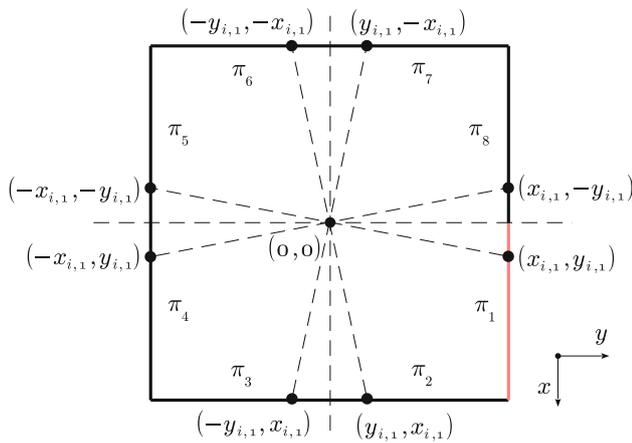
**Fig. 5** Top view of the cuboid projection planes with  $\pi_n$  as the  $n$ th half-plane.  $\pi_1$  is the half-plane calculated in the mapping procedure. The corresponding transformations of an image point  $(x_{i,1}, y_{i,1})$  in  $\pi_1$  to the rest of the half-planes are depicted above
