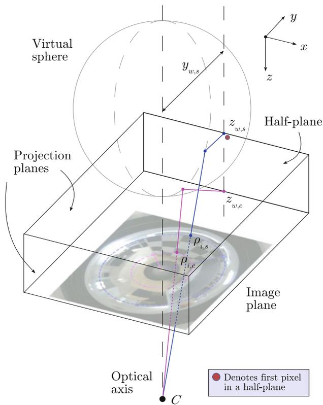
**Fig. 1** The cuboid projection planes can be deduced given that the perpendicular distances of each plane to the optical axis,  $y_{w,s}$ , the vertical start location of each plane,  $z_{w,s}$ , and the corresponding end location,  $z_{w,e}$ , are available. Each projection plane consists of two half-planes that are mirror to each other. The red dot denotes the first pixel location in a half-plane.  $C$  is the centre of projection
