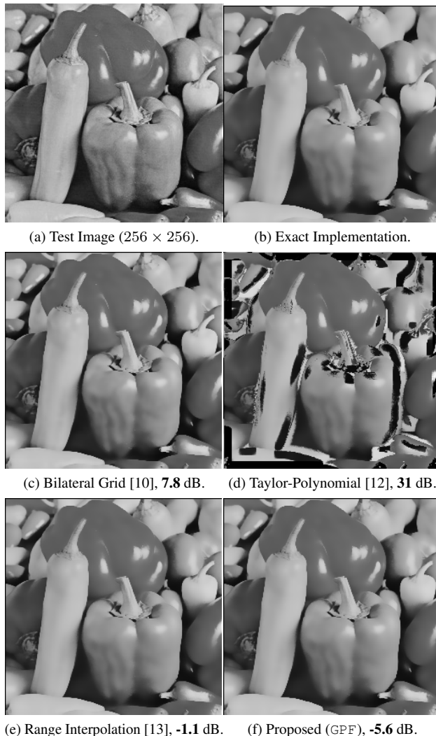
Fig. 4. Comparison of the exact implementation of (1) with various fast algorithms for \sigma_s = 3, \sigma_r = 30 . The degree of the respective functions (raised-cosine, Taylor polynomial, and Gauss-polynomial) used to approximate the range kernel is 20. The MSE between the exact implementation and the various approximations are shown in bold.
