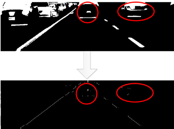
Fig. 5. Drawbacks of the proposed scanning rule: blobs between line markings and outside the current lane.
