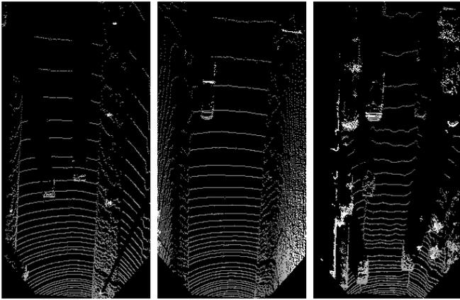
Fig. 1. Three examples of mean elevation images: Each pixel grayscale value encodes the mean elevation of its relative grid cell.
