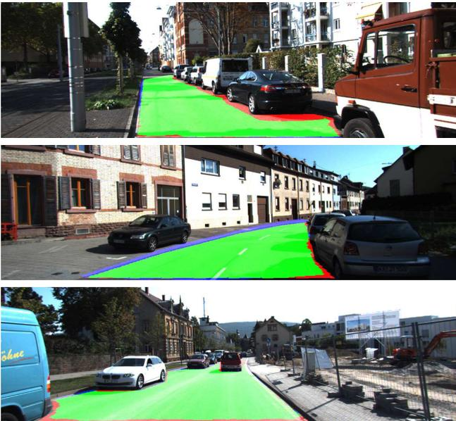
Fig. 5. Examples of road detection in images from the test set. Green denotes true positive; red and blue correspond to false negative and false positive, respectively.
