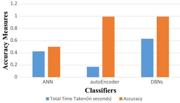
**Figure 9. Time And accuracy measure of different classifiers for epoch value 50.**
