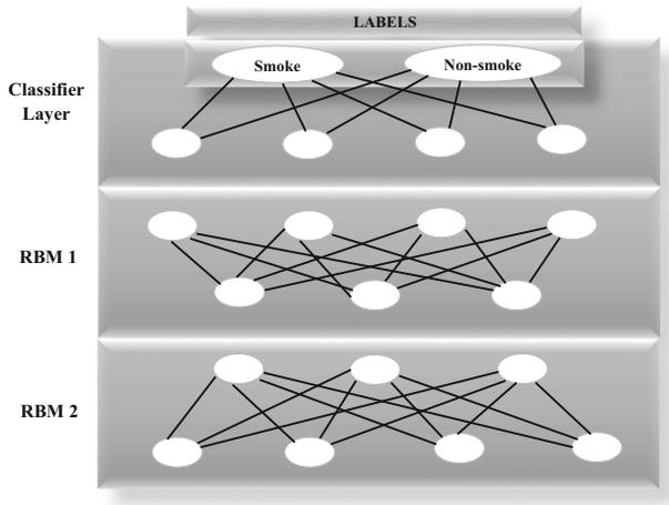
**Figure 3. A DBN classifier with two RBM layers.**
