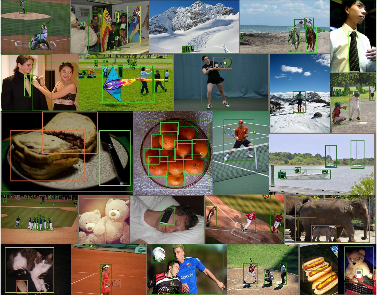
Figure 8 – Some detection results on mini_val split. ResNet-50 is used as the backbone. As shown in the figure, FCOS works well with a wide range of objects including crowded, occluded, highly overlapped, extremely small and very large objects.
