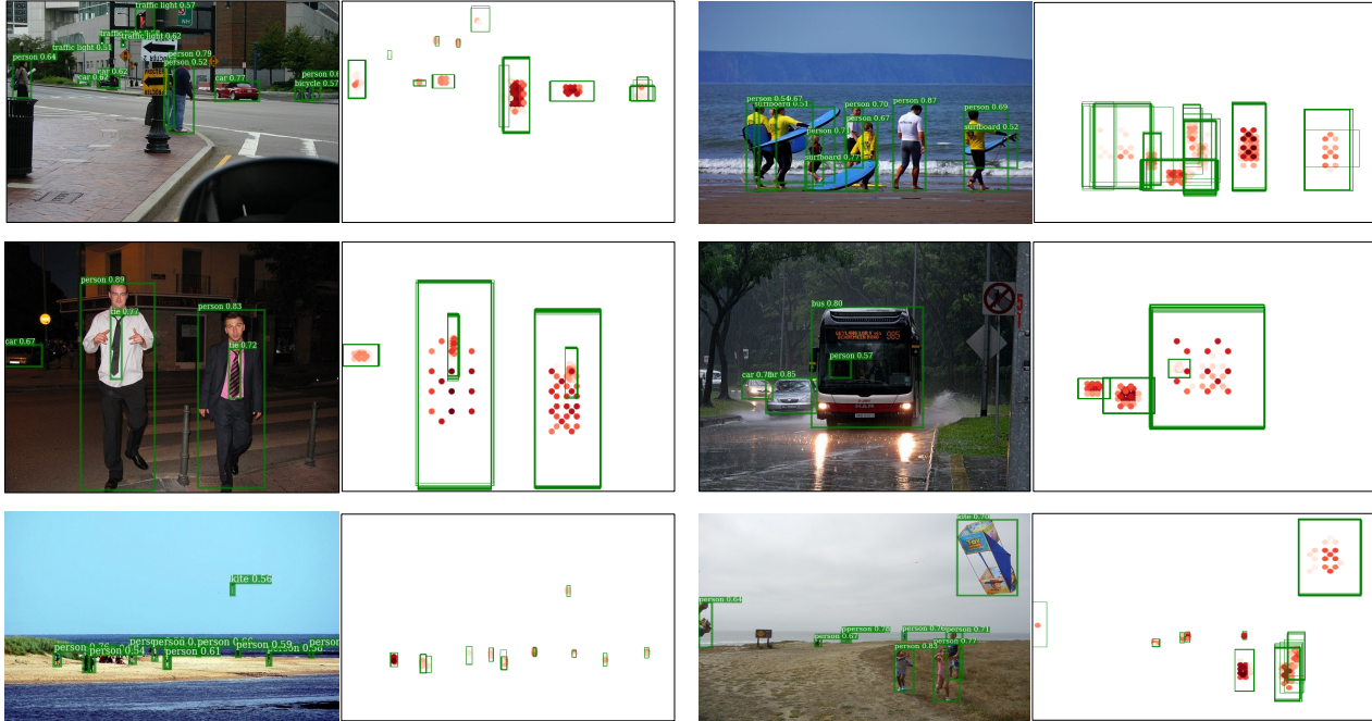
Figure 7. FoveaBox results on the COCO minival set. These results are based on ResNet-101, achieving a single model box AP of 38.9. For each pair, left is the detection results with bounding box, category, and confidence. Right is the score output map with their corresponding bounding boxes before feeding into non-maximum suppression (NMS). The score probability in each position is denoted by the color density. These figures demonstrate that FoveaBox could directly generate accurate, robust box predictions, without the requirement of candidate anchors.
