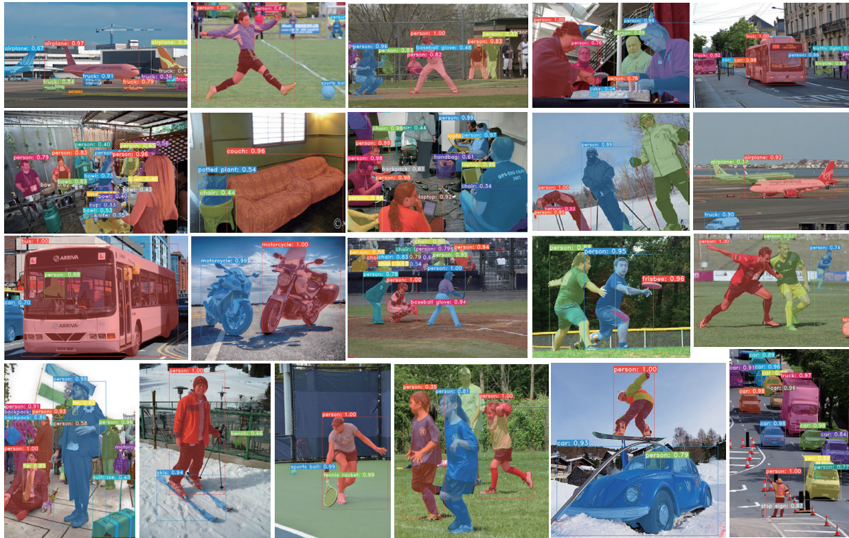
Fig. 7: YOLACT evaluation results on COCO’s test-dev set. This base model achieves 29.8 mAP at 33.0 fps. All images have the confidence threshold set to 0.3.
