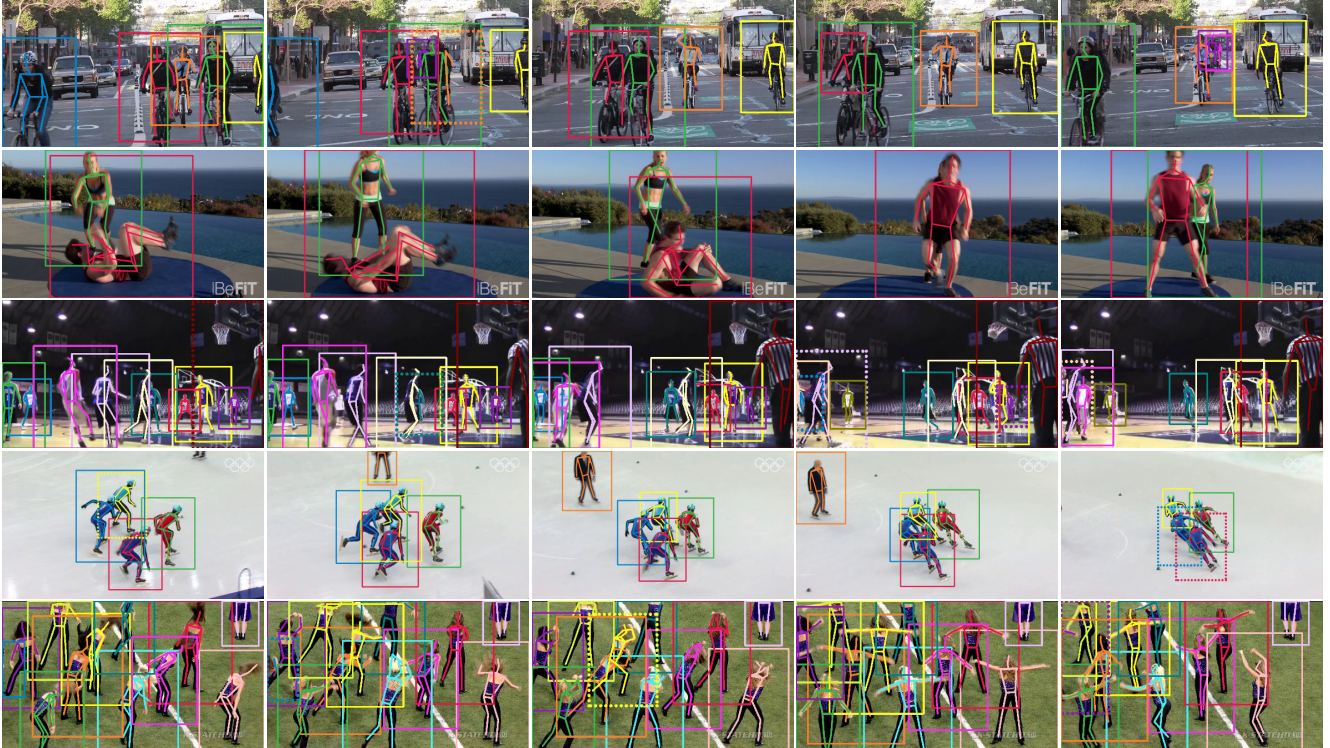
Figure 6: Visualization of the output of our approach on five videos from the PoseTrack dataset. Bounding boxes and poses are color coded using the track id predicted by our model. Solid bounding boxes indicate that the instance was localized by the person detector, while dotted bounding boxes were originally missed by the detector, but recovered by our approach.
