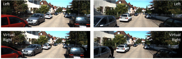
Figure 3. Left image (top) and the generated virtual right image (bottom) using our image-level virtual view generation method.
