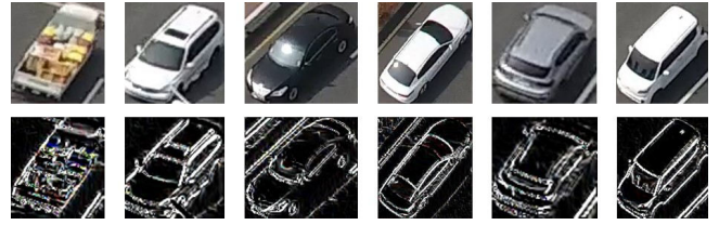
Fig. 3: Within cropped vehicle area to extract edge; first row: cropped image in the original, second row: edge image from a cropped image.
